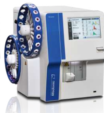
Medonic M32S – Autoloader for up to 2 x 20 samples. Just load and walk away.
